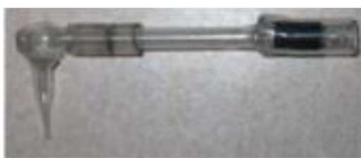
Figure 4. Assembly used to measure catalyst temperature after being removed from the cell shown in Fig. 3. Gas containing a mixture of D_2 and O_2 will form D_2O at the catalyst, seen as the black region in the photograph. The resulting temperature increase is detected by an RTD contained in a sealed Pyrex tube located next to the catalyst. Excess O_2 can leave the cell through a gap between the inner and outer tubes.
