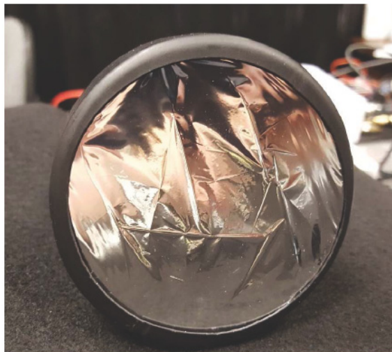
Figure 13. ZnS scintillator/PMT X-ray detector.
