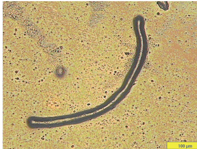
Figure 16. A trail marking on nuclear emulsion. From deuterium glow discharge experiment with W–W cathodes. The scale is 100 \mu\text{m} .
